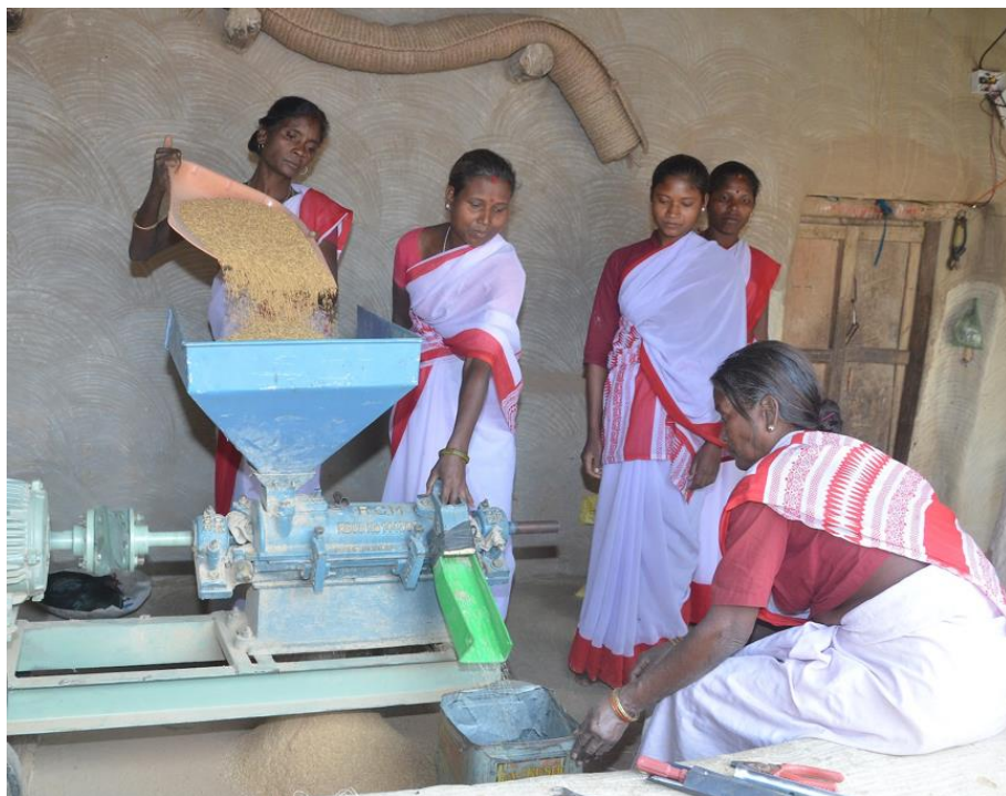
Mini-grids power productive use loads like grain mills Source: Mlinda, 2019
