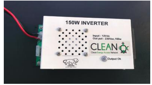
PWM inverter (150 W) without charge controller
