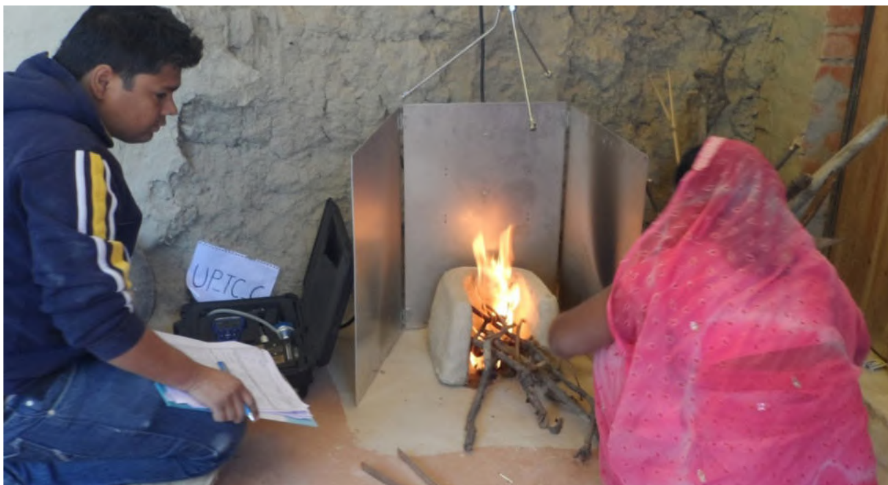
Figure 1. Emissions sampling setup with a Traditional Chulha at the Uttar Pradesh project site location.
